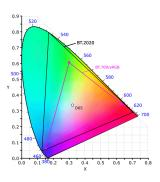
The camera is able to reproduce the extended color space BT.2020 in addition to the BT.709 color space for HDTV. (Prerequisite is a BT.2020 compatible monitor)
